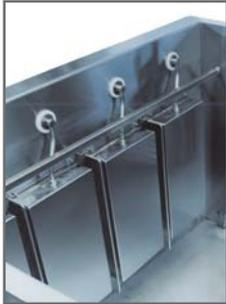
Wall-mounted transducers are often used in applications that release heavy contaminants into the wash solution. Any sludge collecting in the bottom of the tank will not affect their performance.
